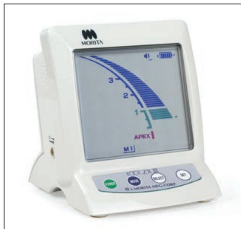
Fig 8-4 A Root ZX electronic apex locator. These units utilize impedance values to accurately measure root canal lengths. Their accuracy is not diminished by apical periodontitis, root resorption, or the presence of irrigants.
